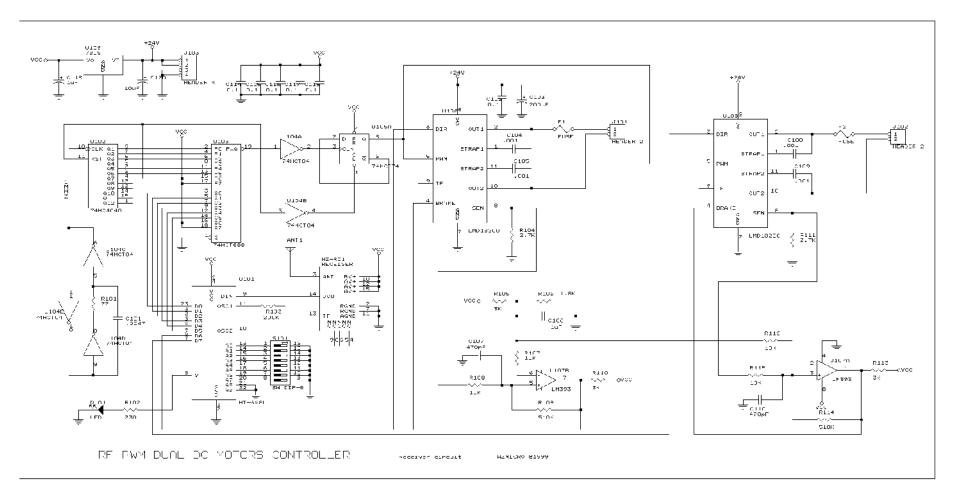
The receiver module WZ-R01 receives the data from the transmitter and feeds that data to the decoder U1 (HT-648L); the 8bit data will then be decoded. The first two significant bits D7 and D6 control the motor rotation direction. The lower 6 bits vary the duty cycle of the output pulse. U2 is a 12bit counter; it is configured so that it will reset itself every 64 counts. The oscillation circuit forms by U4c, U4d and U4e providing approximately 1MHz clock to the counter U2.
