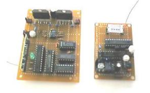
The above picture is the prototype. We had been able to control the motors at more than 100 feet away. It works great!
